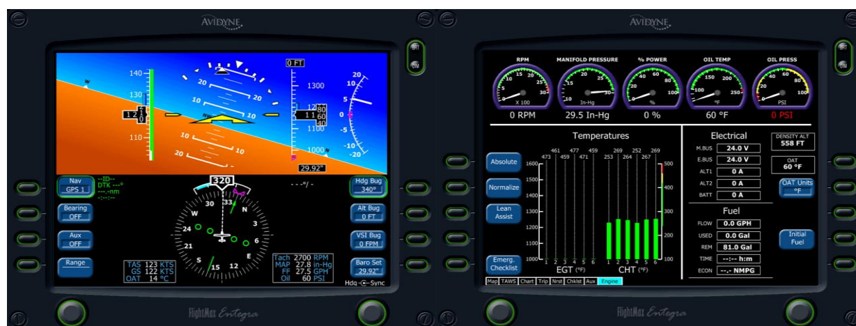
Figure 5: The Avidyne Entegra is similar in functionality to the G1000 (Figure 4) but has a different user interface (Mindstar Aviation, 2016).
