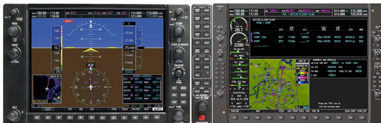
Figure 4: The Garmin G1000 is one of the most popular flight deck systems. The Primary Flight Display (PFD) on the left gives the pilot attitude and control information, such as altitude, heading, and airspeed (NextGA Aircraft, Inc., 2012). The Multi-Function Display (MFD) on the right can be adjusted to the pilot's liking, but tends to display secondary reference information, such as engine data, navigation charts, flight plans, and procedures (Ray, 2013).
